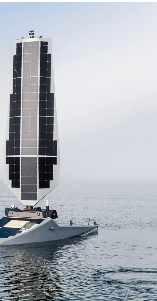
◀ Ocean Aero's 14-ft. Triton autonomous vehicle can be used in defense, scientific, and energy sectors. It collapses the solar panel to submerge
